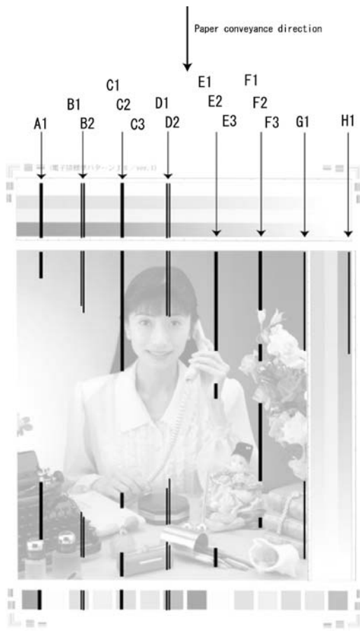
FIG. 16—Graphical comparison between the spur marks on a printout (upper) and on a pressure measurement sheet (lower) for the Canon BJJ800 printer.
